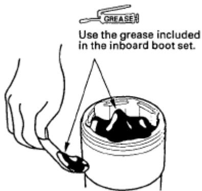
Fig. 101: Packing Inboard Joint With Joint Grease Courtesy of AMERICAN HONDA MOTOR CO., INC.
