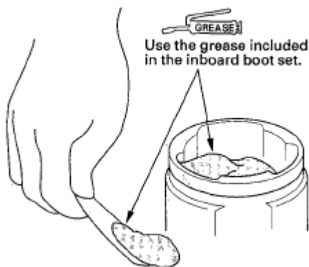
Fig. 31: Filling Inboard Joint With Grease Courtesy of AMERICAN HONDA MOTOR CO., INC.
